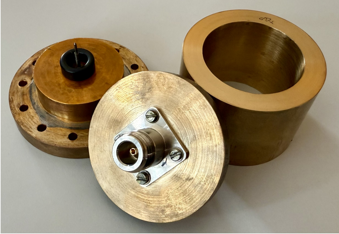
FIG. 1. RF shorted coaxial cell developed within the project.
