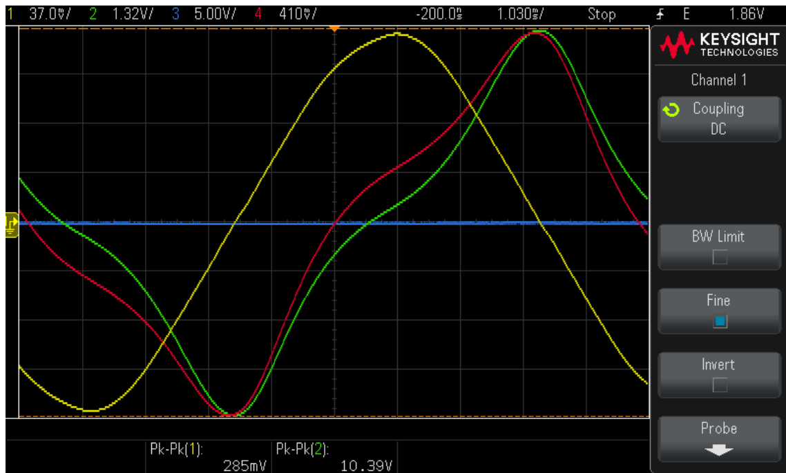
FIG. 3. Oscilloscope screen showing: voltage corresponding to the generated waveform in the arbitrary waveform generator (red), voltage across the calibrated resistor in the primary circuit (green), and the induced sinusoidal voltage in the secondary coil (yellow).
