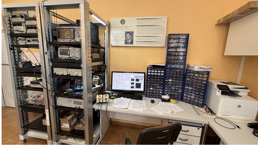
FIG. 2. Hysteresisgraph-wattmeter built in the "Prof. Potocký Laboratory of Ferromagnetism".
